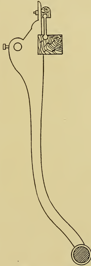
Fig. 49. Lay Sword with Rocker Shaft Connections.
